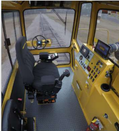
Hercules control panel and operational controls.
