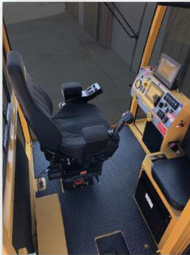
Spartan control panel and operational controls.
