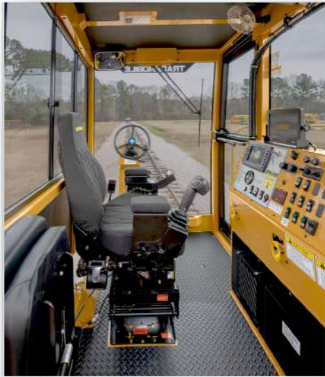
Titan control panel and operational controls.
