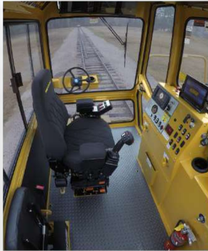
Viking control panel and operational controls.
